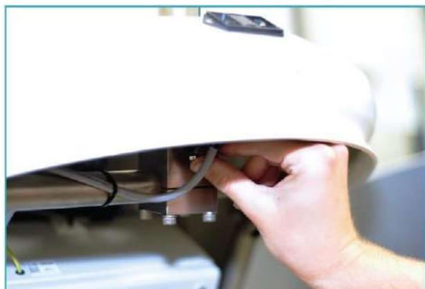
FIXATION AU CUBE AVEC UN ÉCROU PAPILLON
