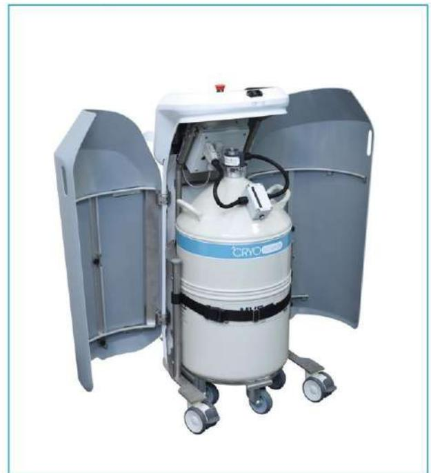
APRÈS LE DÉBALLAGE DE LA MACHINE, PRÉPAREZ LE RÉSERVOIR AU REMPLISSAGE D'AZOTE LIQUIDE. POUR CE FAIRE, OUVREZ LES PORTES ET SUIVEZ LES ÉTAPES CI-DESSOUS. ASSUREZ-VOUS QUE LA TÊTE ET LE FLEXIBLE SONT DÉGIVRÉS AFIN DE NE PAS LES ENDOMMAGER.
